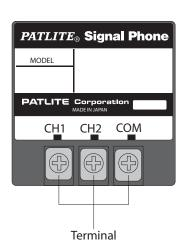
External Contact Capacity: No less than 100mA
